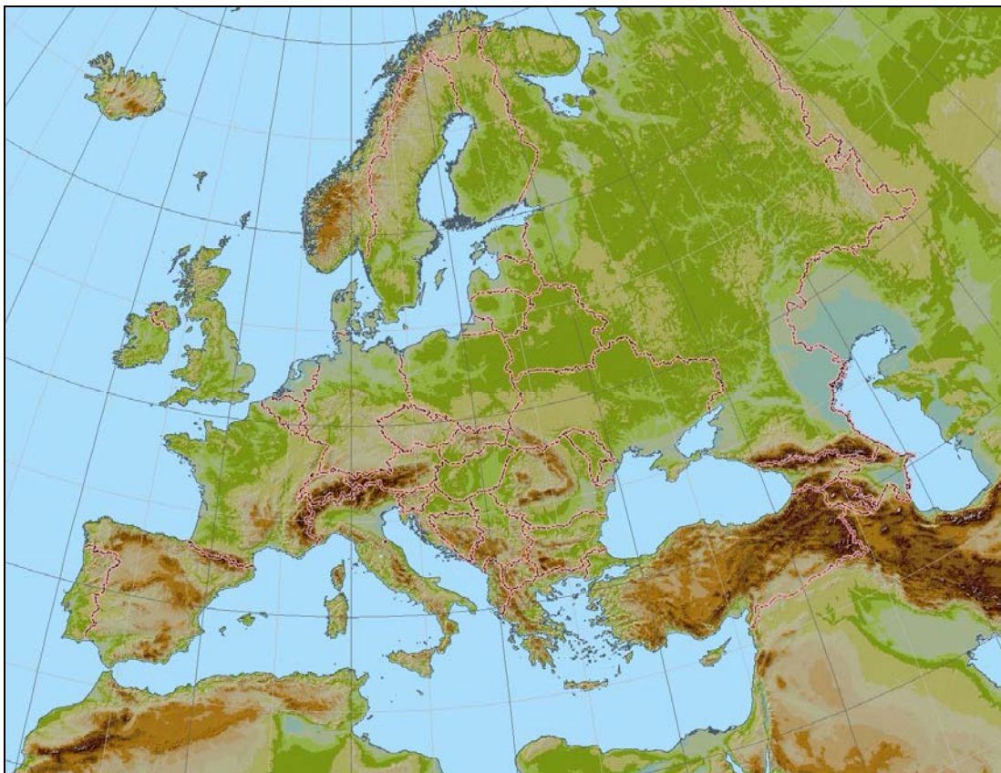
Figure 3: CCM2 Digital Elevation Model. Resulting Mosaic at 100m grid-cell resolution (Atlantic Islands not shown)
